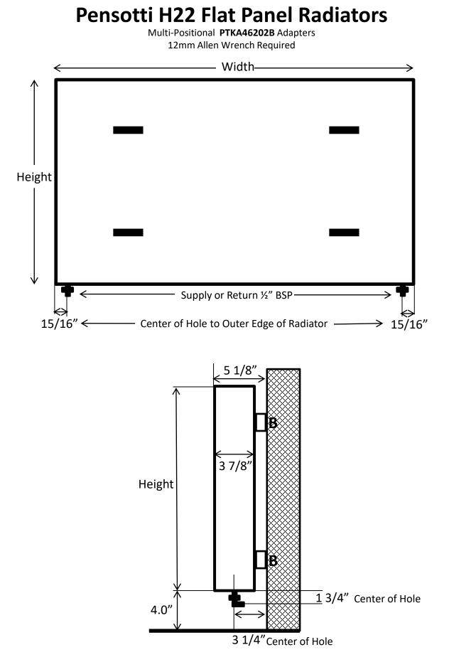
Radiator Mounting Brackets Must Be Secured To Wall Studs Or Proper Wall Backing Material
