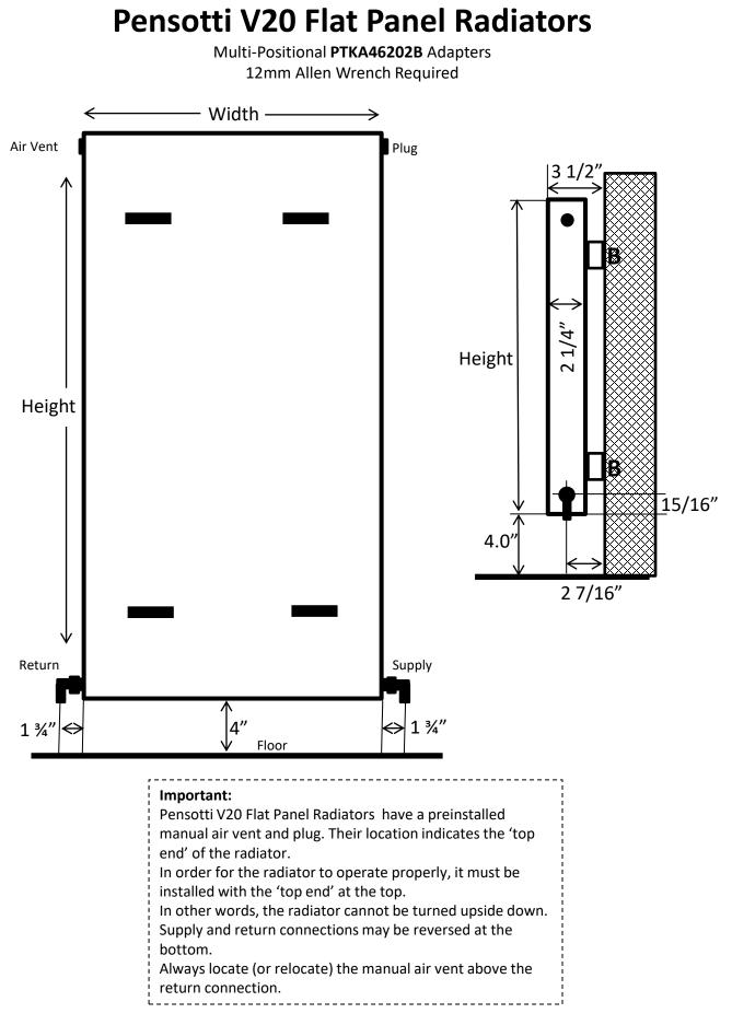
Radiator Mounting Brackets Must Be Secured To Wall Studs Or Proper Wall Backing Material
