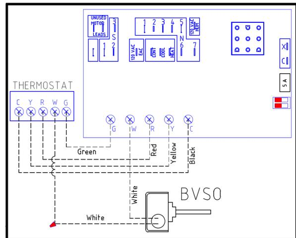
Figure 2 - BVSO wiring diagram
